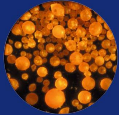
Micro-encapsulated particles of NUQO ® RED
